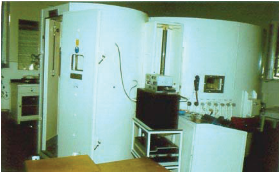
Figure 1. Outside view of an experimental vacuum-chamber equipped with medical measurement devices
