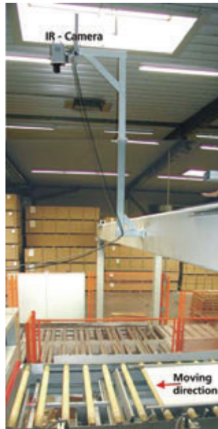
Figure 1: Set-up for passive thermography behind the press
