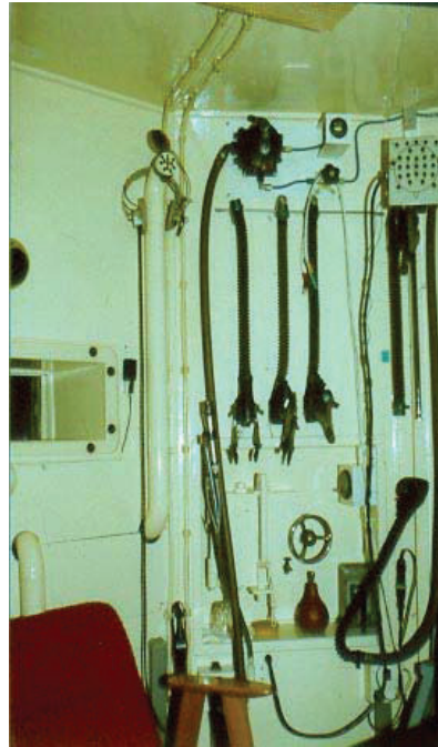
Figure 3. Inside view in the vacuum-chamber with oxygen respiration equipment
