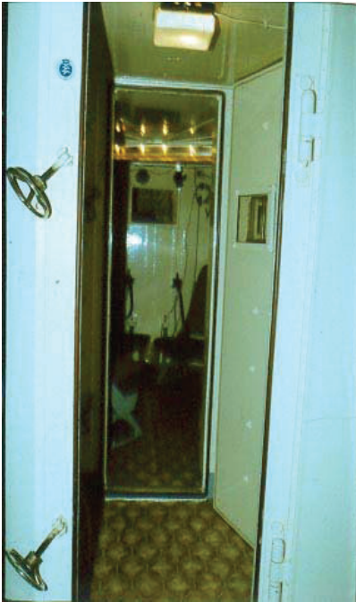
Figure 2. Lock-chamber of the main vacuum-chamber for sluicing/locking successive pressure equalising
