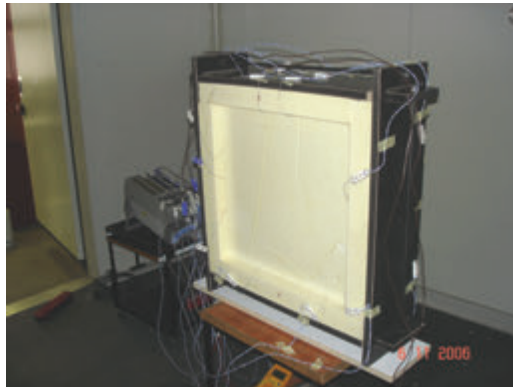
Figure 3. The test rig for prefabricated panel
